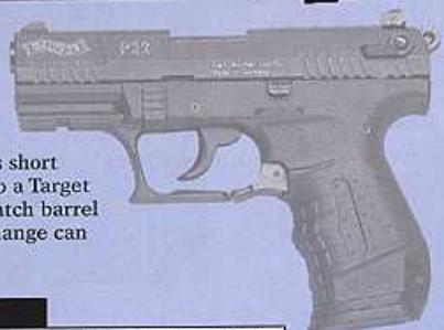
The P22 Standard with its short barrel can be converted to a Target version with a 127 mm match barrel and barrel weight. This change can be performed in seconds.
