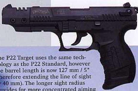
The P22 Target uses the same technology as the P22 Standard, however the barrel length is now 127 mm / 5" (therefore extending the line of sight by 40 mm). The longer sight radius provides for more concentrated aiming during target shooting, ergo resulting in better scores. The P22 Target also is equipped with barrel weight / non functional compensator.
